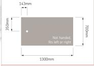
Tray with gravity waste code: 16013W Tray with upward pump waste code: 16100 Tray only code: 16013
