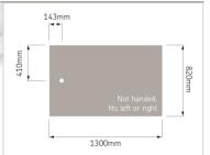
Tray with gravity waste code: 16050W Tray with upward pump waste code: 16141 Tray only code: 16050
