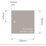
Tray with gravity waste code: 16470W Tray with upward pump waste code: 16471 Tray only code: 16470
