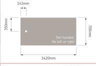
Tray with gravity waste code: 16022W Tray with upward pump waste code: 16109 Tray only code: 16022
