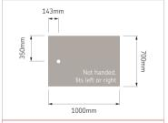
Tray with gravity waste code: 16000W Tray with upward pump waste code: 16083 Tray only code: 16000
