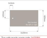
Tray with gravity waste code: 16058W Tray with upward pump waste code: 16150 Tray only code: 16058
